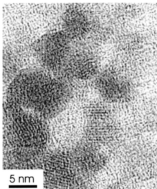
FIG. 2. TEM of NZFO nanoparticles.
